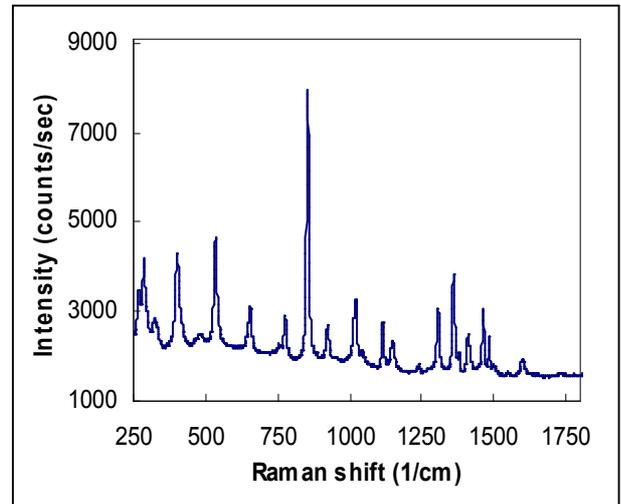
Figure 1: Typical Raman spectral fingerprint.
