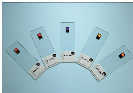
Klarite test slides used for biomarker trace analysis
