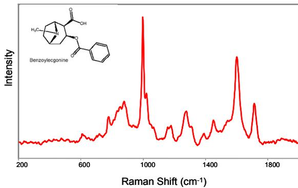
Fig 2. Trace spectra of 1 femtogram of cocaine metabolite benzoylcegonine recorded in 15 sec
