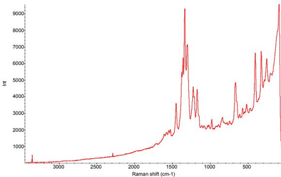
Fig 1. Raman signal of Inkjet printer ink extracted from paper
