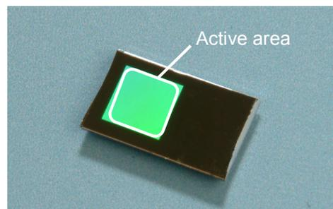
Figure 2: SERS active area on Klarite onto which sample should be deposited
