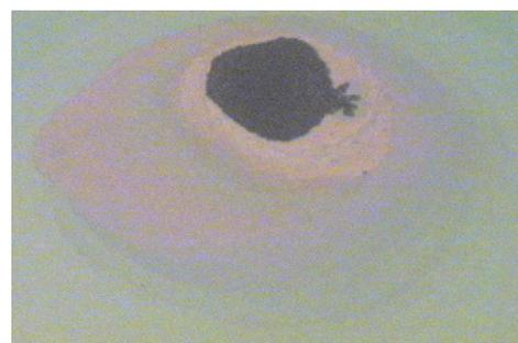
Figure 3: Evaporated drop of a 5mM L-Alanine on Klarite recorded with a 5x microscope objective.
