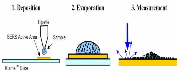
Figure 1: Standard Klarite deposition
