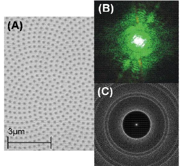
Illustration of a proprietary Sunflower Photonic Quasicrystal designed for far-field emission in the green. (A) SEM of the proposed design (B) Out-of-plane far field emission highlighting the narrow cone light projection (C) Diffraction pattern of the quasicrystal indicating the circular Bragg peaks.
