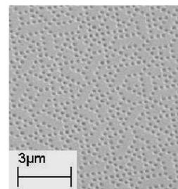
SEM micrograph of a high order symmetry Pinwheel Photonic Quasicrystal structure defined using a selection of tiling rules showing the complex non-periodic orientation of the pattern.
