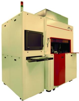
Molecular Imprints produces imprint lithography systems capable of reproducibly mass-producing sub 50nm features on a range of substrates and materials.
