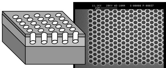
A Photonic Crystal designed for controlling visible light emission is illustrated on the left. The associated scanning electron microscope image of a fabricated device is shown alongside. Typical features are 100's nm in size.
